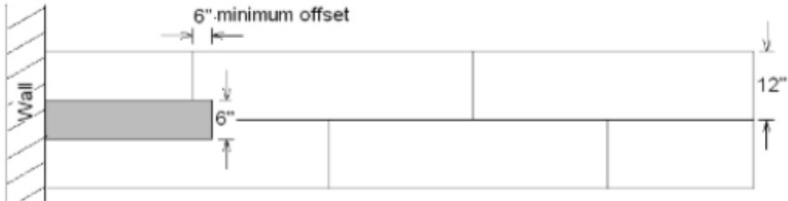
DIAGRAM 3 – OFFSET THE PLANK AND UNDERLAYMENT JOINTS BY AT LEAST 6" (15 CM).
